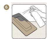
Now, Thibra can be painted with acrylic paint or varnish. For maximum adhesion, prime with spray paint. It is also possible to lightly sand Thibra before painting.
