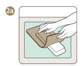
Cover an object with the heated material. Evenly press Thibra onto the surface. You can use your hand or sculpting tools to copy the details of the underlying object.
