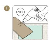
Cover surface with a silicone mat. Heat Thibra with a hot air gun on medium, the material will become flexible and soft. Best deformable at 70 °C. Careful: the material is too hot when it becomes shiny.
